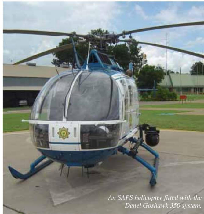
An SAPS helicopter fitted with the Denel Goshawk 350 system.
