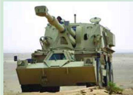
In a continuing drive to improve its acknowledged lead in tubed artillery systems, Denel shattered all previous artillery records by firing 75km earlier this year. This range improvement was achieved on 11 April 2006 with the latest G6-52L, Denel's extended range version of its renowned G6 self-propelled artillery system. It fired V-LAP projectiles which use both base-bleed and rocket-assist technology to extend the range.
