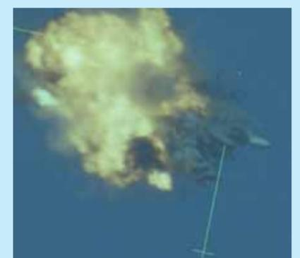
This spectacular photograph records a bitter sweet moment. It shows the destruction of one of our own by one of our own - a Denel Skua target drone by a live Umkhonto surface to air missile launched from the SAS Spioenkop (more on page 2). The test took place at Denel's Overberg Test Range in less than favourable conditions (significant wind and wave action) and at an intercept range exceeding the design requirement by 15%.
